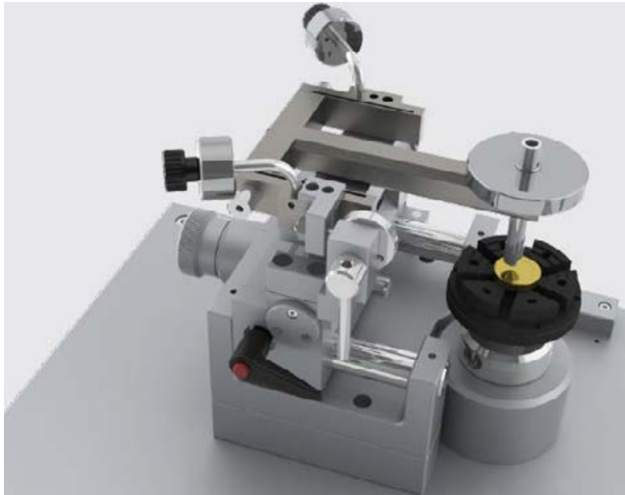
Figure 1: Anton Paar pin-on-disk tribometer fortesting up to 400°C.
