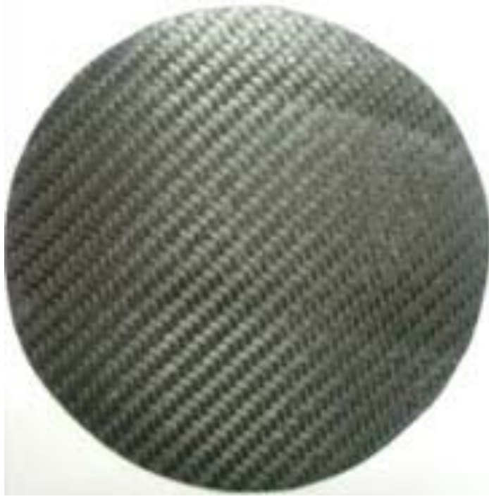
\Phi 111 \times 2 mm thickness test piece for forming
