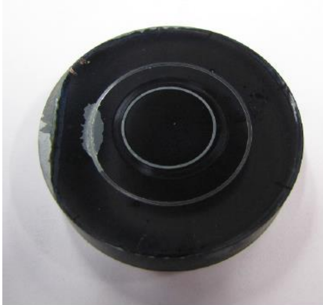
Figure 7: Image of the wear track on the TiAlN coating after the 24°C and 600°C tests. Note area with extensive damage to the coating where oxidation of the substrate occurred.
