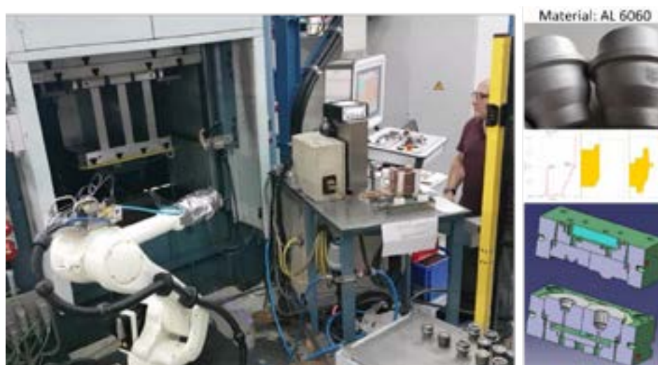
Figure 1: Model factory, fully automated and digitalized two-stage hot forging of Al6060.
