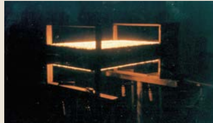
As Faces Radiantes “Iluminam” homogeneamente as ferramentas
