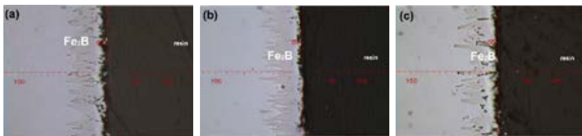
Fig.3. Micrographs of the boride layer of the AISI 1045 specimens treated at 1173 K for 4 h, (a) Nd-boronized, (b) Sm-boronized and (c) Gd-boronized.
