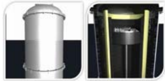
Figure 10 – Crucible of the Czochralski method
