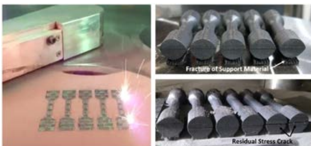
Figure 4: Crack development in L-PBF tensile test samples manufactured with a zero-rotation angle relative to the base plate
