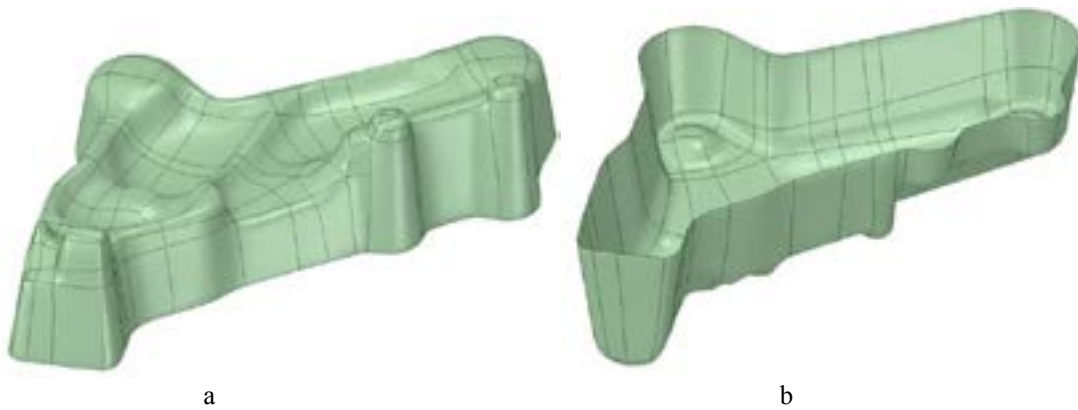
Fig. 3. The equipotential surfaces generated by QForm Direct and used for the creation of the upper (a) and the bottom (b) preforming dies cavities.
