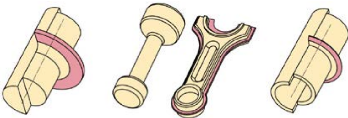
Figure 2 Schematic representation of bulk forming parts exhibiting regions (refer to the pink color) where material flow takes place under plane stress conditions (solid rod flange, connecting rod and tube flange).
