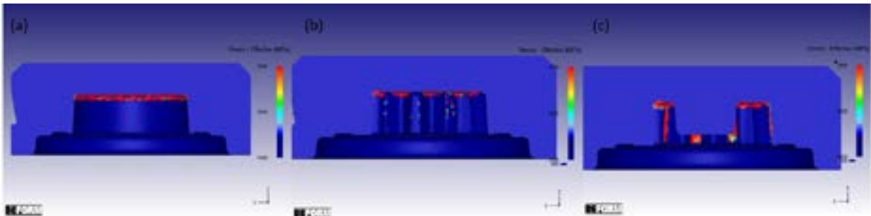
Figure 10: Comparison of effective stress in MPa (with a lateral view): a) Actual top die, b) Top die with teeth, c) Top die with punch.
