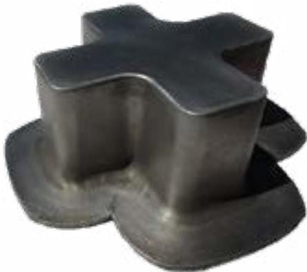
**Fig. 12:** Hot Die Forming “HDF” standard cross sample produced by hot gas forming of a high-strength aluminum alloy with material replenishment (drawing depth 45 mm).
