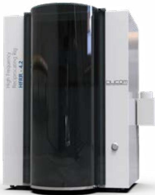
**Figura 4.4.** Tribômetro do tipo *High Frequency Reciprocating Rig* (HFRR 4.2).
