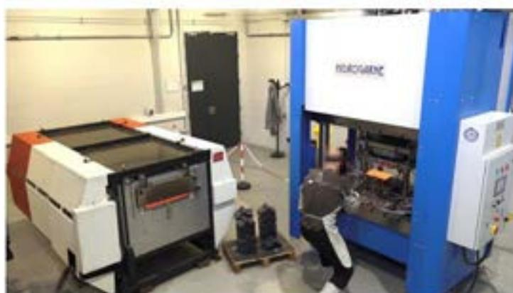
Figure 1. Lab-scale hot stamping plant.
